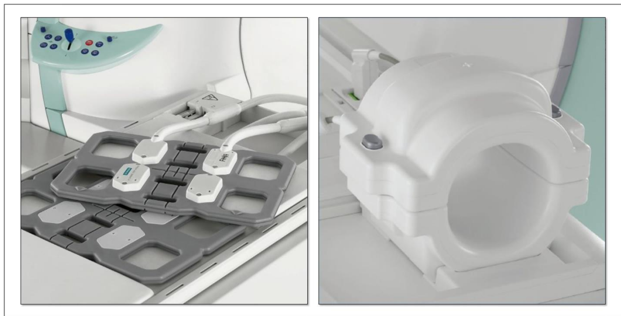
Figure 4-4 Siemens 6 Channel Body Coil (left panel). [103] This coil facilitated scanning of both knees with the full diagnostic and morphological protocol while keeping scan session to 1 hour in duration. It was used for all scanning time points except 168 days postoperative, or the post-euthanasia scan session. Siemens 15 Channel Knee Coil (right panel). [104] This coil was used to scan one knee at a time at the 168 days postoperative time point. For these scans, 1 hour was allocated per knee.
